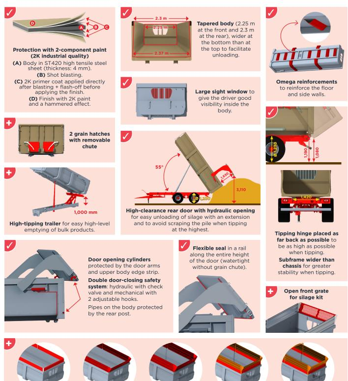
Extensions of 300 (steel or aluminum), 500 (aluminum) or 700 mm (aluminum), stackable up to 1 m. To limit weight and facilitate assembly by a single person: 2-part side extensions on single- and double-axle models, and 3-part extensions on triple-axle models.
